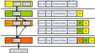
Figure 6 ABA processing sequence
